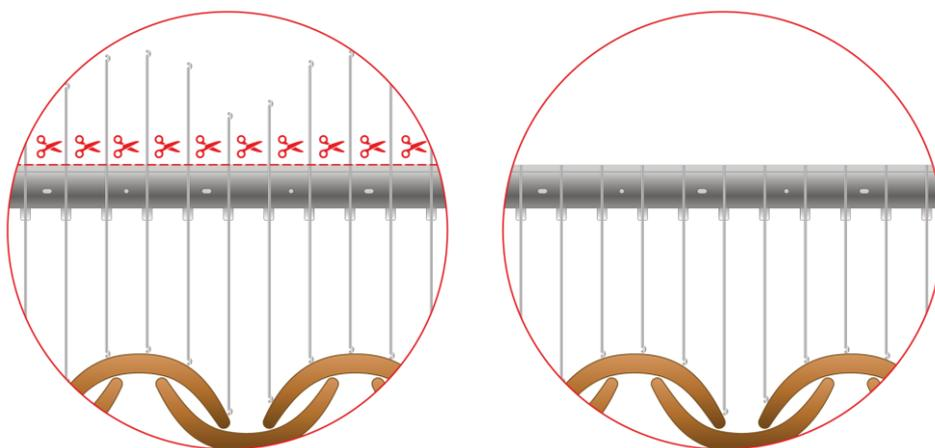
In this way, the snow can slide smoothly without being stopped by protruding segments that could create an impediment to its natural sliding. The snow could subject the protruding barrier to excessive pressure and under the weight of the snow itself, enveloping it and detaching it from the frame of the photovoltaic panels.
