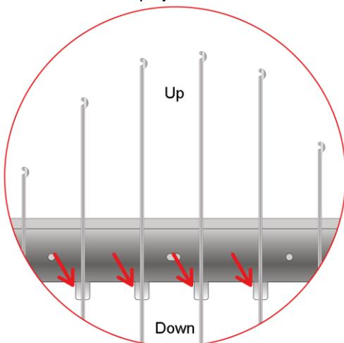
**3.7.2** Use the lower edge of the aluminium frame of the photovoltaic panel as a reference to support the barrier and apply it (see example below).
