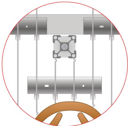
Dedicated templates are present in the package which precisely indicate the positions in which to place the barrier. This precise positioning will allow optimal installation of the barrier under the profiles in order to obtain perfect closure of the compartment. (see example below)
