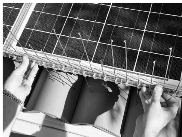
**N.B.!** The rod-type segments will begin to descend autonomously due to the effect of gravity, sliding inside their anchorage seats until they rest on the underlying cover in a uniform manner. In the event that some segments do not descend independently, lightly press with your hands on the top of the same filaments until they reach their end of travel near the cover (see example below)
